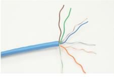
**STEP 5**Separate each wire pair by untwisting.
