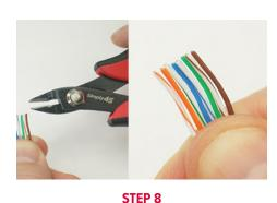
Using a flush cutter, trim the wires straight across so all of the wires are the same length.
