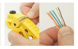
**STEP 6**Straighten each wire conductor.
