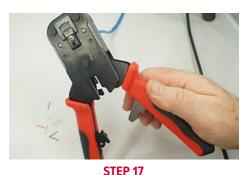
If the crimper handles do not release this means that you have not completed the crimping cycle. Simply squeeze the crimper handles further down until the crimper handles release.
