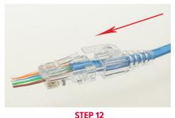
If using strain relief/boot, slide the boot up and into the back of the plug until the boot clip covers the top of the plug clip.
