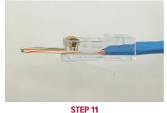
Push the plug as far down onto the cable until it stops inside the plug.
